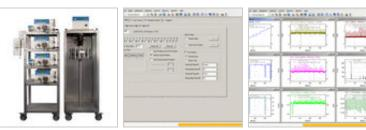
The SMB System CSEP C9812 Production Unit is designed for the extraction of pure substances in kilogram-scale. Special emphasis is put on the continuous operation mode and high productivity.
